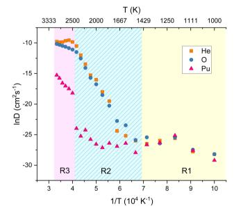
Fig. 2 Diffusivity as a function of temperature for helium, oxygen and plutonium in PuO<sub>2</sub>. 0.5% He concentration, simulation evolved for 5 ns at every 100 K between 1000-3000 K. Helium and oxygen diffusivity are closely linked. Plutonium diffusion begins at approx. 2500 K. Three regions R1, R2 and R3 are highlighted which are explained in the text.
