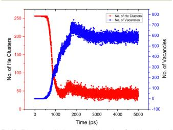
Fig. 13 The number of helium clusters (left y-axis, red) and the number of Pu and O vacancies (right y-axis, blue) as a function of time. The simulation was of PuO<sub>2</sub> at 2250 K with a 4% He concentration. As the number of vacancies increases, the number of clusters decreases, as more helium atoms are joining clusters so the overall number decreases as there are fewer, bigger helium clusters. After 3000 ps a stable state of the number of He clusters and lattice vacancies is established
