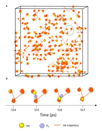
Fig. 5 Trajectories of He atoms in initially defect-free PuO<sub>2</sub> at 2100 K. (a) Displays the trajectory of all He atoms over a period of 1 ns. (b) Displays a snapshot of an inter-site hop by a He atom from the area circled in green in (a). The time period in (b) is 514-517 ps. It can be seen that at 515 ps an oxygen vacancy is generated in the vicinity of the helium and the helium uses this to migrate to a neighbouring OIS.
