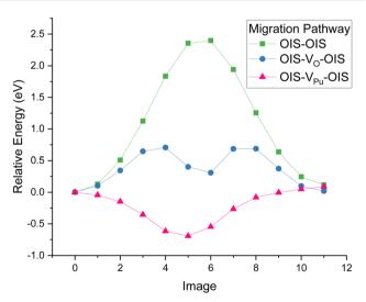
Fig. 1 Relative energy barriers for different migration pathways for He to move between two interstitial sites in PuO<sub>2</sub> from NEB calculations. A direct OIS-OIS hop (green squares) has the highest energy barrier, migrating via an oxygen vacancy (blue circles) has a much lower energy barrier and via a plutonium vacancy (pink triangles) there is a negative energy at the plutonium vacancy site, so this site may act as a trap for helium rather than a migration pathway
