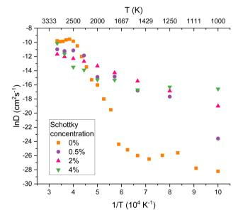
Fig. 6 Helium diffusivity as a function of temperature for four different Schottky defect concentrations in PuO<sub>2</sub>. The helium concentration was 2% with all helium atoms initially randomly inserted into OISs. One can see that He diffusion occurs even at low temperatures when Schottky defects are present.
