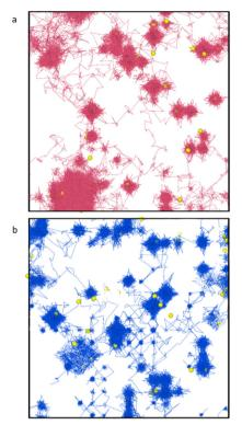
Fig. 8 Trajectory of helium atoms in PuO2 with a 2% Schottky defect concentration at 2250 K over 1 ns. (a) Displays the trajectory when the helium atoms started in V<sub>Pu</sub> sites (pink lines) and (b) when the helium started in V<sub>O</sub> sites (blue lines). There is much less interstitial site hopping when helium atoms are input at plutonium vacancies
