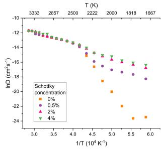
Fig. 7 Oxygen diffusion coefficients as a function of temperature in PuO<sub>2</sub> at four different Schottky defect concentrations. Below the phase change at approx. 2500 K the concentration of defects has a significant effect on oxygen diffusivity. In the superionic phase, the diffusivity of oxygen is the same for all Schottky concentrations, as at these temperatures the oxygen sublattice is amorphous.
