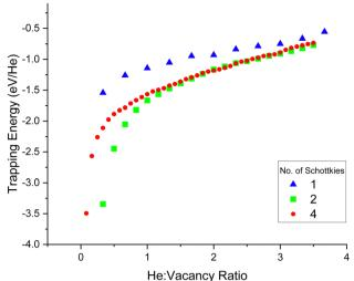
**Fig. 10** Trapping energies of He atoms at Schottky void sites as a function of a cluster's He: vacancy ratio. A more negative trapping energy means a more energetically favourable site for helium to occupy. Three seed locations for the clusters were considered, made of 1, 2 and 4 Schottky defect clusters.
