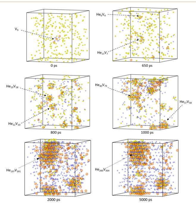
Fig. 15 PuO<sub>2</sub> supercell with 4% He concentration at 2250 K. Initially three Schottky trios (V<sub>Pu</sub> pink spheres, V<sub>O</sub> blue spheres) were input in the centre of the lattice with the He atoms (yellow spheres) randomly inserted in OISs. Cluster formation shown at different times and the He: vacancy ratios labelled.
