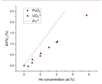
Fig. 3 Percentage volume expansion as a function of the helium concentration in PuO<sub>2</sub>, UO<sub>2</sub> and Pu. <sup>a</sup> Yun et al. <sup>46 b</sup> Wolfer. <sup>9</sup> Experiments show a typical volume expansion of 1% after large irradiation doses (Helen Steele, private communication) indicating a maximum He concentration of 5%.
