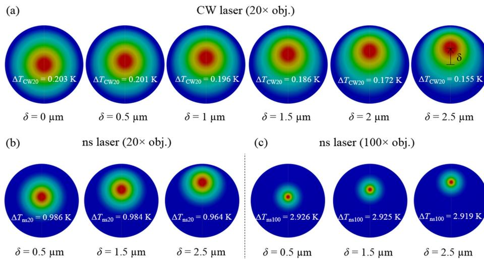
Fig. 10 Results of numerical analysis conducted by Zobeiri *et al.* to investigate the effect of laser spot position on the uncertainty of measured  $D$  of a suspended  $\text{WS}_2$  film. (a) CW laser heating ( $20\times$ ), (b) ns laser heating ( $20\times$ ), and (c) ns laser heating ( $100\times$ ). Reproduced from ref. 34 with permission from Elsevier, copyright 2019.
