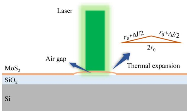
Fig. 4 Thermal expansion of the MoS<sub>2</sub> film on the SiO<sub>2</sub> substrate under laser irradiation.
