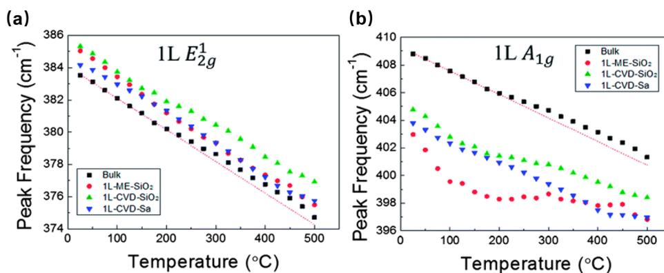
Fig. 3 Temperature dependence of the two Raman modes of monolayer MoS<sub>2</sub>: (a) E<sub>2g</sub><sup>1</sup> and (b) A<sub>1g</sub>. Reproduced from ref. 30 with permission from the Royal Society of Chemistry, copyright 2014.
