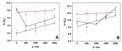
Fig. 4 Pressure dependence of the binding constant, K<sub>b</sub>, for the complex formation between the ligand proflavine and (A) BSA and (B) HSA in 20 mM Tris-HCl buffer, pH 7.4 (black squares) and in buffer containing 0.5 M TMAO (red circles) and 0.5 M GB (blue triangles) at T = 25 °C. From the slope of  $ln(K_b)$  vs. p, the binding volume,  $\Delta V_b$ , was obtained.
