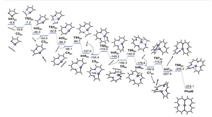
Fig. 5 Same as Fig. 3a, but for the Phot0 pigment from the intermediate Int1<sub>Zn</sub>.
