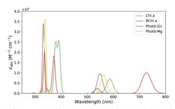
Fig. 2 Theoretical UV/Vis absorption spectra of Chl a (green), BChl a (red), Phot0-Mg (yellow) and Phot0-Zn (purple) in vacuum. Phytyl groups of Chl a and BChl a are substituted by a methyl group
