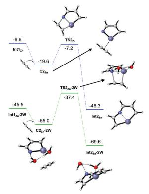
Fig. 4 Same as Fig. 3a, but for the formation of the intermediates Int2<sub>Zn</sub> and Int2zn-2W
