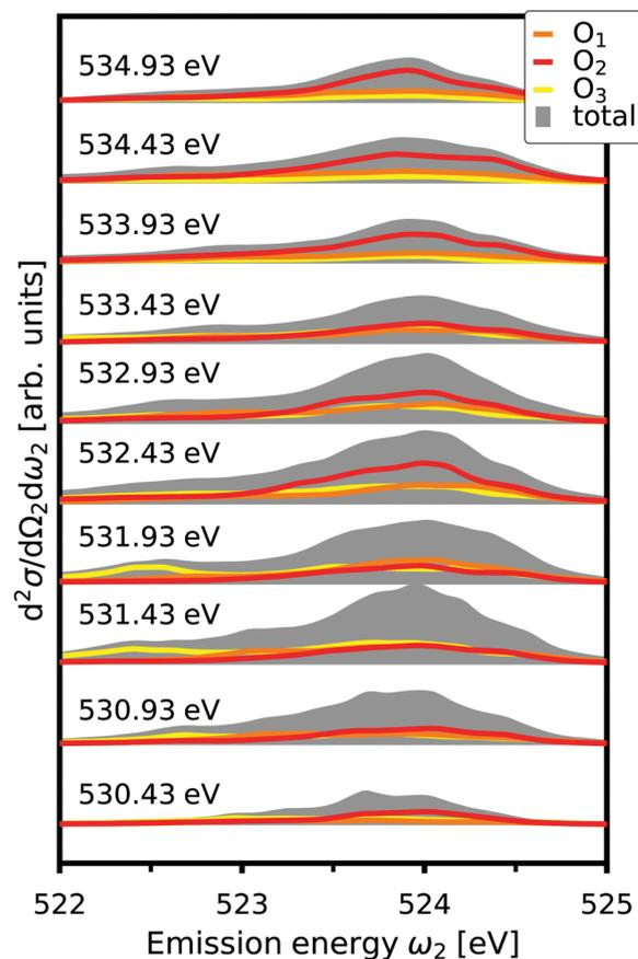
Fig. 3 Total O K edge RIXS in  $\beta$ - $\text{Ga}_2\text{O}_3$  as a function of emission energy,  $\omega_2$ , for selected excitation energies, together with the contributions from  $\text{O}_1$ ,  $\text{O}_2$ , and  $\text{O}_3$ . The spectra are offset for clarity.
