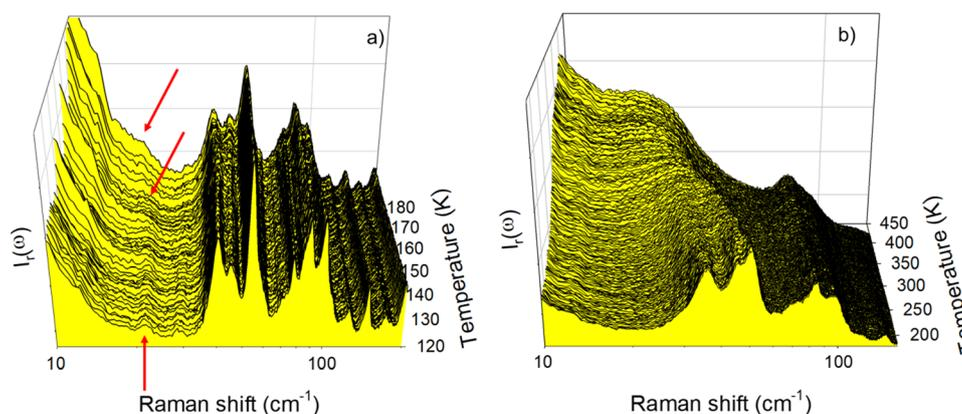
Fig. 2 Low-frequency Raman spectra of L-Nle collected upon heating from 120 K at  $1 \text{ K min}^{-1}$  plotted by step of 1 K (a) in the 120–180 K temperature range, (b) in the 180–450 K temperature range; arrows show the soft mode.
