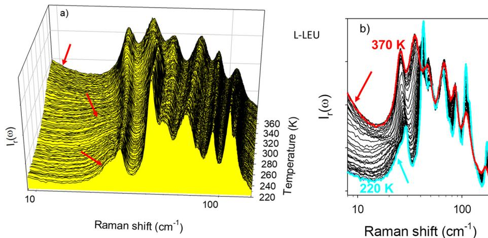
Fig. 1 Low-frequency Raman spectra of L-LEU collected upon heating from 220 K at  $1 \text{ K min}^{-1}$ , (a) plotted by step of 1 K, (b) plotted by step of 5 K, arrows are used to show the temperature behavior of the soft mode.
