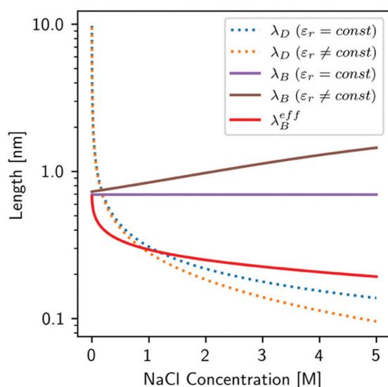
Fig. 16 The effect of varying the relative permittivity ( $\epsilon_r$ ) due to concentration on both the Debye length ( $\lambda_D$ ) and the unscreened Bjerrum length ( $\lambda_B$ ), as well as the predicted effective (or screened) Bjerrum length ( $\lambda_B^{\text{eff}}$ ).
