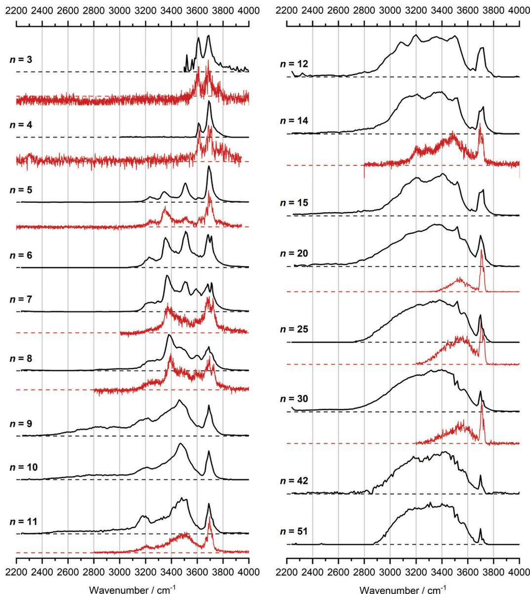
Fig. 1 Infrared multiple photon dissociation spectra of the  $V^+(H_2O)_n$  complexes ( $n = 3-12, 14, 15, 20, 25, 30, 42$  and  $51$ ) presented in black. For comparison, infrared spectra from Duncan and coworkers are also presented in red for cluster sizes  $n = 3-5, 7, 8, 11, 14, 20, 25$  and  $30$ .<sup>62</sup>
