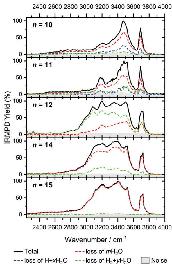
Fig. 7 Infrared multiple photon dissociation spectra of  $V^+(H_2O)_n$  complexes ( $n = 10-12, 14, 15$ ). In each case photodissociation events are due to sequential loss of either (i) loss of intact water molecules  $mH_2O$ , (ii) loss of  $H + xH_2O$ , and (iii) loss of  $H_2 + yH_2O$ , represented as dashed red, blue, and green lines, respectively.
