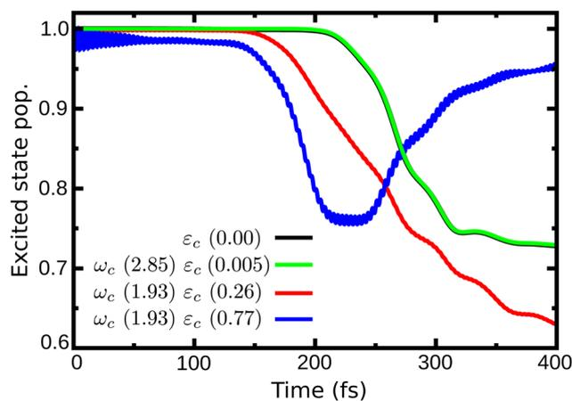
Fig. 4 Time dependent population in the excited state for case (1) ( $\omega_c = 2.85$  eV,  $\varepsilon_c = 0.005$  GV m<sup>-1</sup>), case (2) ( $\omega_c = 1.93$  eV,  $\varepsilon_c = 0.26$  GV m<sup>-1</sup>) and case (3) ( $\omega_c = 1.93$  eV,  $\varepsilon_c = 0.77$  GV m<sup>-1</sup>).
