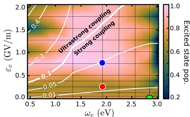
Fig. 3 Population in the excited state, at 400 fs, as a function of the cavity resonance frequency  $\omega_c$  and field strength  $\varepsilon_c$ . The coupling strength ( $g_{ij}/\omega_c$ ) is shown by the contour lines. The colored dots mark the position of the cases considered in Fig. 4 and in the discussion.
