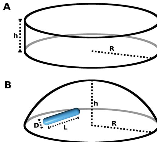
Fig. 1 Schematic depiction of the confinement considered in our simulation of three-dimensional liquid crystals. We simulate the liquid crystals by a system of  $N$  spherocylinders with length  $L$  and diameter  $D$  in confinement to suppress the bulk symmetry of the fluid in order to observe topological defects. (A) Cylindrical cavity with radius  $R$  and height  $h$ . (B) Spherical-cap cavity with radius  $R$  and height  $h$ .
