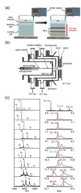
Fig. 3 (a) Schematic illustration of PAGE separation techniques. 61 (b) Details of the ESI source. (c) Negative-ion ESI mass spectrum of each fraction separated by PAGE. <sup>102</sup> In right figure,  $Au_n(SG)_m$  is described as n-m. Reproduced with permission from ref. 61 and 102. Copyright 2020 The Royal Society of Chemistry and 2005 American Chemical Society.
