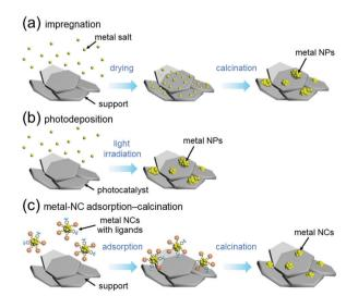
Fig. 13 Comparison of (a) impregnation, (b) photodeposition, and (c) metal-NC adsorption—calcination methods.
