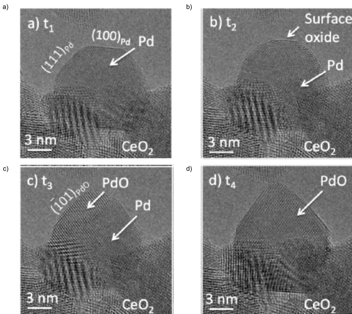
Fig. 4 High resolution ETEM observation of Pd to PdO transformation at oxygen partial pressure of ~1 mbar and temperature of 400 °C. (a) Initial Pd nanoparticle supported on CeO<sub>2</sub>. (b) Transition period corresponding to the formation of surface oxide. (c) Transition period corresponding to growth PdO. (d) Final stage of transformation corresponding to the formation of PdO. Adapted with permission from ref. 115.
