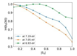
Fig. 8 The PES is fitted by three Gaussian in order to extract the electron yield in the 3d channel as a function of  $|S_3|$ , for different two-photon excitation energies. For each energy, the electron yield is normalized to its own maximum
