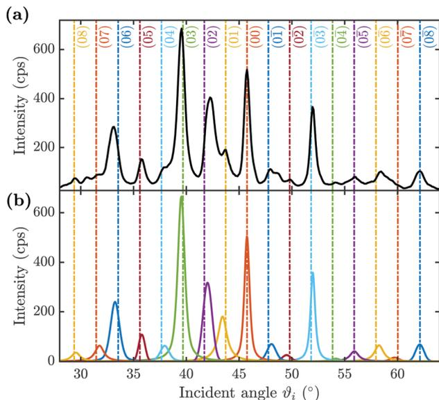
Fig. 3 (a) Characteristic  $\theta$ -scan of the Bi(114) surface along  $\overline{110}$  (measured data shown by the black line) with the sample temperature kept constant at  $T_s = 114$  K. The energy of the incident helium beam was held constant at  $E_i = 10.58$  meV. The coloured vertical lines represent the theoretically calculated peak positions with the corresponding  $\mathbf{G}$ -vectors. (b) Fits of the measured diffraction peaks using a scaled pseudo-Voigt profile.
