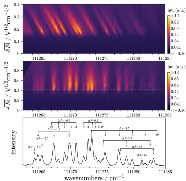
**Fig. 6** Experimental measurement of the  $X^{+2}\Pi_{g,1/2}(v^+ = 0) \leftarrow X^1\Sigma_g^+(v = 0)$  transition of CO<sub>2</sub> recorded with the PRFI-ZEKE method. The linearized matrix, the rotated matrix, and the final spectrum are depicted in the upper, middle, and lower panels respectively. The color scales are arbitrary. The final spectrum has been obtained by integrating the rotated matrix over the  $y$  range delimited by the white dotted lines.
