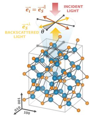
Fig. 2 Schematic of the Raman scattering polarization measurements. Raman measurements are performed on (001) basal plane with incident laser light (wide red arrow) projected along the z-axis ([001] direction). The incident light polarization and the output polarization in perpendicular configuration are represented by the thin red and yellow arrows, respectively. The black arrows indicate the x and y axis of the crystal corresponding to [100] and [010] directions, respectively
