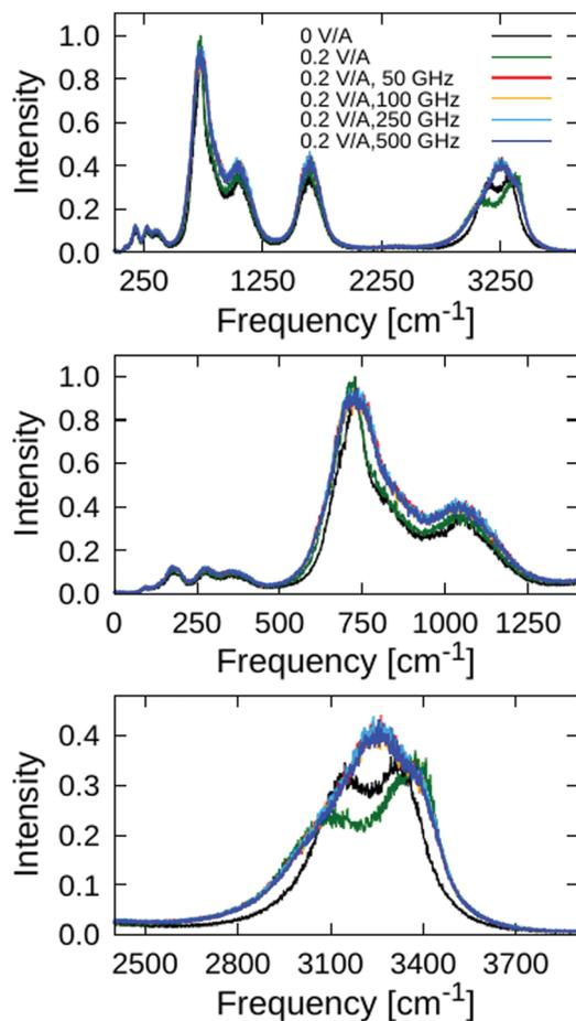
Fig. 5 Vibrational density of states (VDOS) obtained by Fourier transform of the velocity autocorrelation function. Effect of the static and oscillating electric fields of magnitude  $0.2 \text{ V \AA}^{-1}$  is shown compared to the zero-field spectrum (labeled as  $0 \text{ V \AA}^{-1}$ ). The whole spectrum is plotted in the upper panel while the librational and stretching bands are shown in detail in the middle and lower panels, respectively.
