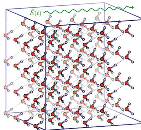
Fig. 1 Structure of proton-ordered ice VII model used in the simulations. The cubic supercell of side length  $12.62 \text{ \AA}$  contains 128 water molecules. Direction of the applied oscillating electric field is indicated by green arrow.
