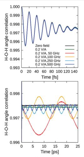
Fig. 3 Autocorrelation function (ACF) of H-O-H valence-angle bending vibrations shown at a short-time scale of the first 150 fs (left) and longtimescale of 25 ps (right). Field effects of static as well as alternating applied electric fields are compared with the zero-field ACF curve (plotted in black).
