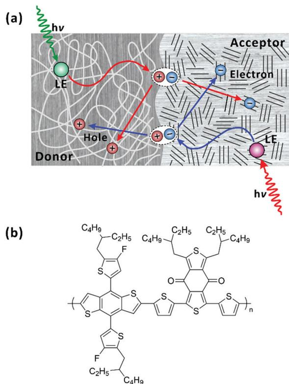
**Fig. 1** (a) Simplified illustration of photophysical processes in bulk-heterojunction organic photovoltaic devices. In both donor and acceptor domains, when locally excited (LE) states are generated upon photoexcitation, the LE states diffuse to the donor–acceptor interface and form charge-transfer state (CT). The CT state dissociates across the donor–acceptor interface into charge-separated states. (b) Chemical structure of PM6.
