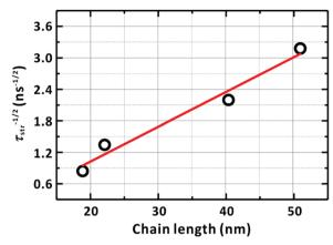
Fig. 10 Dependence of the diffusion time of the LE/CT state on the chain length. The diffusion time is assumed to be identical to the average lifetime  $(\tau_{\text{str}})$  in Table 4 of the LE/CT state. The solid line represents the linear relationship between  $\tau_{\rm str}^{-1/2}$  and the chain length, l. The PM6 chain length was estimated by multiplying the reported length of a PM6 repeating unit (1.54 nm) by the degree of polymerization of each sample; see ref. 57.
