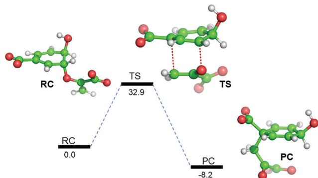
Fig. 3 B3LYP/Def2-SVP gas-phase energy profile diagram for the inter-conversion of chorismate to prephenate. The energies are reported in kcal mol<sup>-1</sup> relative to the reactant complex (RC).
