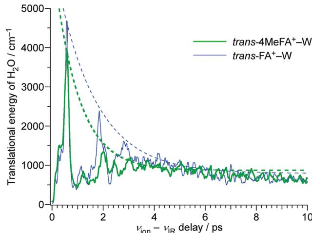
Fig. 10 Time profiles of the kinetic energy change in the water molecule of the *trans*-4MeFA<sup>+</sup>-W and *trans*-FA<sup>+</sup>-W obtained by the MD simulation. Single exponential curves representing the decay of the energy are shown as dashed lines. The damping time constants are 0.96 ps for 4MetFA<sup>+</sup>-W and 1.53 ps for tFA<sup>+</sup>-W.
