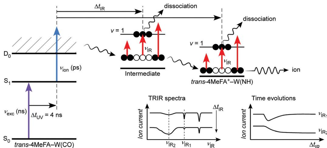
Fig. 2 Excitation scheme of the ns excitation–ps ionization–ps IR time resolved spectroscopy. A single vibronic level in the excited state, which is prepared precisely by the ns excitation pulse ( $\nu_{\text{exc}}$  (ns)), is ionized by  $\nu_{\text{ion}}$  (ps) to trigger solvent dynamics in the cationic  $D_0$  state, and the dynamics is probed by the tunable  $\nu_{\text{IR}}$  (ps) pulse through time-resolved IR photodissociation spectroscopy.
