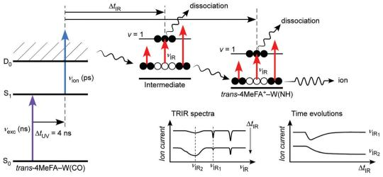
Fig. 2 Excitation scheme of the ns excitation-ps ionization-ps IR time resolved spectroscopy. A single vibronic level in the excited state, which is prepared precisely by the ns excitation pulse ( $\nu_{\text{exc}}$  (ns)), is ionized by  $\nu_{\text{ion}}$  (ps) to trigger solvent dynamics in the cationic D<sub>0</sub> state, and the dynamics is probed by the tunable  $\nu_{IR}$  (ps) pulse through time-resolved IR photodissociation spectroscopy.
