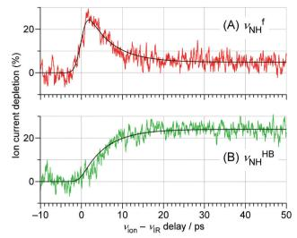
Fig. 7 TEs probed at the (A)  $\nu_{\rm NH}^{\rm f}$  (3393 cm<sup>-1</sup>) and (B)  $\nu_{\rm NH}^{\rm HB}$  (3200 cm<sup>-1</sup>) vibrations of trans-4MeFA+-W obtained by the ns-excitation-psionization scheme (Fig. 6). The best fits obtained by the kinetic analysis are also shown. The background signal in (A) after 30 ps arises from the tail of the strong  $v_{\rm NH}^{\rm HB}$  band. See Section S-13 in ESI† for the detained explanation of the fitting model.
