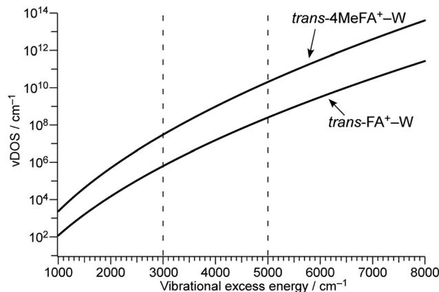
Fig. 9 Vibrational excess energy dependence of vibrational density of states (vDOS) of *trans*-4MeFA<sup>+</sup>-W and *trans*-FA<sup>+</sup>-W. In *trans*-4MeFA<sup>+</sup>-W, contributions from the CH<sub>3</sub> internal rotation are estimated regarding the CH<sub>3</sub> groups as independent rotors. Dashed lines indicate the excess energy range (3000–5000 cm<sup>-1</sup>) of the product P<sup>+</sup> after photoionization.
