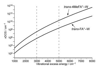
Fig. 9 Vibrational excess energy dependence of vibrational density of states (vDOS) of trans-4MeFA<sup>+</sup>-W and trans-FA<sup>+</sup>-W. In trans-4MeFA<sup>+</sup>-W, contributions from the CH<sub>3</sub> internal rotation are estimated regarding the CH<sub>3</sub> groups as independent rotors. Dashed lines indicate the excess energy range (3000-5000 cm<sup>-1</sup>) of the product P<sup>+</sup> after photoionization.
