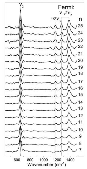
Fig. 2 Experimental IRMPD spectra of  $[Cu_n,CO_2]^+$  (n=7-25) in the 400–1500 cm<sup>-1</sup> spectral range (the line a five-point adjacent-average). Dashed vertical lines are shown as guide to the eye.
