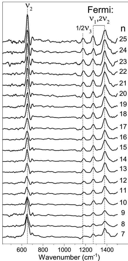
Fig. 2 Experimental IRMPD spectra of  $[\text{Cu}_n\text{CO}_2]^+$  ( $n = 7-25$ ) in the 400–1500  $\text{cm}^{-1}$  spectral range (the line a five-point adjacent-average). Dashed vertical lines are shown as guide to the eye.
