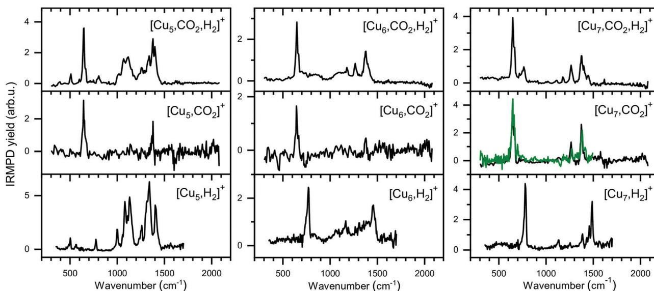
Fig. 8 Experimental spectra of [Cu<sub>n</sub>, CO<sub>2</sub>, H<sub>2</sub>]<sup>+</sup>, [Cu<sub>n</sub>, CO<sub>2</sub>]<sup>+</sup>, and [Cu<sub>n</sub>, H<sub>2</sub>]<sup>+</sup> for n = 5–7 presented in a similar manner as for the Cu<sub>4</sub><sup>+</sup> complexes in Fig. 6. The green trace on the [Cu<sub>7</sub>, CO<sub>2</sub>]<sup>+</sup> spectrum is the reference spectrum from Fig. 3 obtained during individual CO<sub>2</sub> adsorption experiments.
