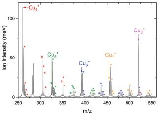
Fig. 4 Mass spectrum of  $[Cu_n, mCO_2, pH_2]^+$  with n = 4-8, m = 0-2, and p = 0-4 obtained using isotopically enriched <sup>65</sup>Cu. Masses corresponding to complexes are color-coded according to the color of the bare cluster. The hash tag (#) indicates attachment of CO<sub>2</sub> and the asterisk (\*) of H<sub>2</sub>.
