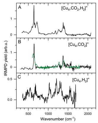
Fig. 5 Experimental IRMPD spectra of  $[Cu_4, CO_2, H_2]^+$  (A) and  $[Cu_4, CO_2]^+$ (B, black). Panel B also shows the [Cu<sub>4</sub>, CO<sub>2</sub>]<sup>+</sup> reference spectrum from Fig. 3E (green trace), and Panel C that for [Cu<sub>4</sub>, H<sub>2</sub>]<sup>+</sup> from ref. 50.
