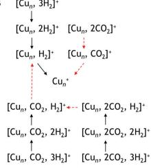
Scheme 1 Observed fragmentation pathways. Pathway A is observed for  $Cu_4^+$  pathway B for  $Cu_5^+$ ,  $Cu_6^+$ ,  $Cu_7^+$ . Black solid arrows indicate  $H_2$  loss, red dashed arrows  $CO_2$  loss.
