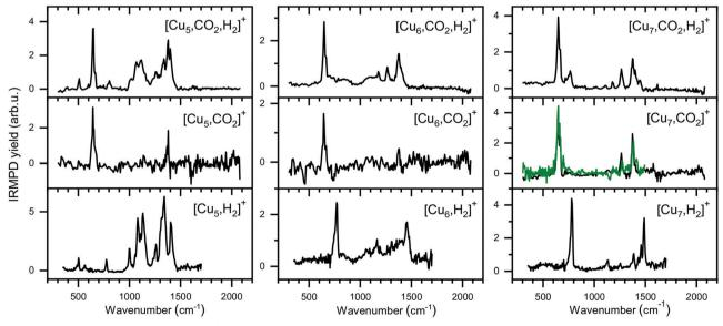
Fig. 8 Experimental spectra of  $[Cu_n, CO_2, H_2]^+$ ,  $[Cu_n, CO_2]^+$ , and  $[Cu_n, H_2]^+$  for n = 5-7 presented in a similar manner as for the  $Cu_4^+$  complexes in Fig. 6. The green trace on the [Cu<sub>7</sub>, CO<sub>2</sub>]<sup>+</sup> spectrum is the reference spectrum from Fig. 3 obtained during individual CO<sub>2</sub> adsorption experiments
