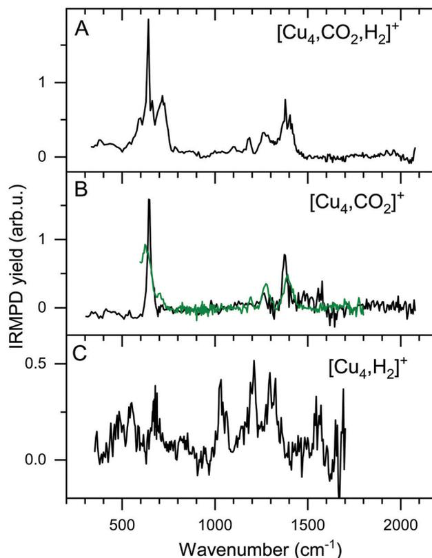
Fig. 5 Experimental IRMPD spectra of  $[\text{Cu}_4, \text{CO}_2, \text{H}_2]^+$  (A) and  $[\text{Cu}_4, \text{CO}_2]^+$  (B, black). Panel B also shows the  $[\text{Cu}_4, \text{CO}_2]^+$  reference spectrum from Fig. 3E (green trace), and Panel C that for  $[\text{Cu}_4, \text{H}_2]^+$  from ref. 50.
