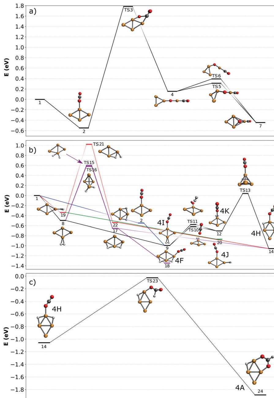
Fig. 7 Potential energy surfaces describing adsorption reactions on  $\text{Cu}_4^+$ . (a)  $\text{CO}_2$  adsorption and dissociation; (b) co-adsorption of  $\text{H}_2$  and  $\text{CO}_2$  (color codes are used to identify different pathways in the text; dashed lines denote simplified pathways for which full path are shown in the ESI<sup>†</sup>); (c)  $\text{CO}_2$  reduction to formate. All energies are given with respect to the reactants.
