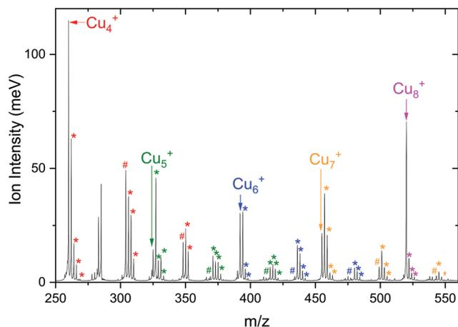
Fig. 4 Mass spectrum of  $[\text{Cu}_n, m\text{CO}_2, p\text{H}_2]^+$  with  $n = 4-8$ ,  $m = 0-2$ , and  $p = 0-4$  obtained using isotopically enriched  $^{65}\text{Cu}$ . Masses corresponding to complexes are color-coded according to the color of the bare cluster. The hash tag (#) indicates attachment of  $\text{CO}_2$  and the asterisk (\*) of  $\text{H}_2$ .
