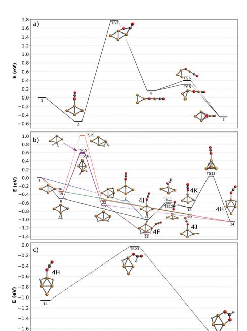
Fig. 7 Potential energy surfaces describing adsorption reactions on  $Cu_4^+$ . (a)  $CO_2$  adsorption and dissociation; (b) co-adsorption of  $H_2$  and  $CO_2$  (color codes are used to identify different pathways in the text; dashed lines denote simplified pathways for which full path are shown in the ESI†); (c)  $CO_2$  reduction to formate. All energies are given with respect to the reactants.
