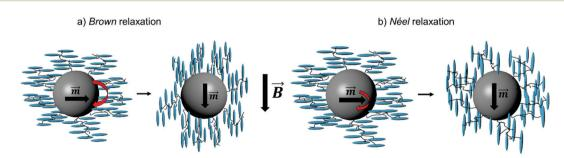
Fig. 1 Possible relaxation mechanism of nanoparticles in a magnetic field: Brown and Néel relaxation.
