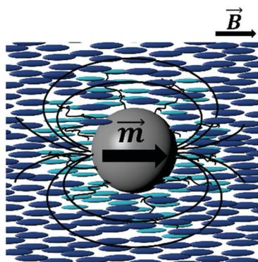
**Fig. 10** Schematic illustration of a LC polymer-decorated magnetic nanoparticle in a LC host matrix and an applied external field. The covalently bond polymer brush is partly swollen with host mesogens.
