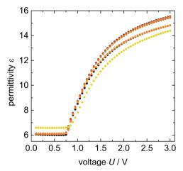
Fig. 8 Permittivity  $\varepsilon$  as a function of electric field for 5CB ( $\bullet$ ) and 9OCB-PHMS@Fe<sub>3</sub>O<sub>4</sub> doped 5CB with different magnetic volume fraction  $\phi_{\rm m}$  =  $1.9 \times 10^{-5}$  (**()**),  $\phi_{\rm m} = 9.4 \times 10^{-5}$  (**()**),  $\phi_{\rm m} = 1.9 \times 10^{-4}$  (**()**),  $\phi_{\rm m} = 4.7 \times 10^{-4}$ (**a**) and  $\phi_{\rm m} = 9.4 \times 10^{-4}$  (**b**).
