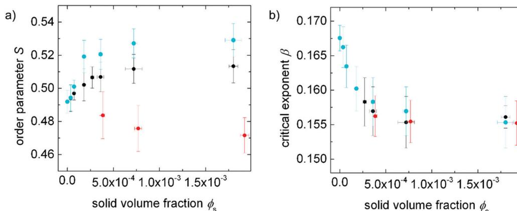
Fig. 7 (a) Order parameter at a reduced temperature of  $\tau = 0.985$  and (b) critical exponent  $\beta$  as a function of solid volume fraction  $\phi_s$  for 5CB doped with 9OCB-PHMS@Fe<sub>3</sub>O<sub>4</sub> (●), 9OCB-PHMS@CoFe<sub>2</sub>O<sub>4</sub> (●), and 9OCB-PHMS@SiO<sub>2</sub> (●). The values for 9OCB-PHMS@CoFe<sub>2</sub>O<sub>4</sub> and 9OCB-PHMS@SiO<sub>2</sub> are taken from ref. 21.
