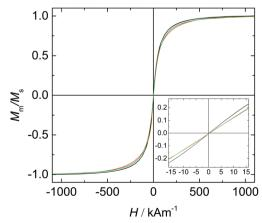
Fig. 4 Magnetization curves of a dried CA@Fe<sub>3</sub>O<sub>4</sub> particles (-), CA@Fe<sub>3</sub>O<sub>4</sub> particles dispersed in water (-) and 9OCB-PHMS@Fe<sub>3</sub>O<sub>4</sub> particles in 5CB (-).
