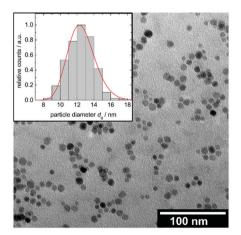
Fig. 3 TEM image and corresponding size histogram of CA@Fe<sub>3</sub>O<sub>4</sub> nanoparticles with a log normal distribution function (-).
