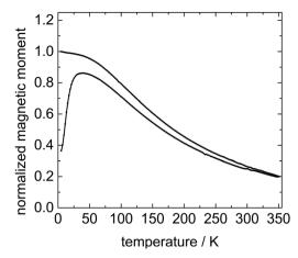
Fig. 5 Normalized ZFC-FC magnetization curves recorded at 10 mT for 9OCB-PHMS@Fe<sub>3</sub>O<sub>4</sub> in 5CB
