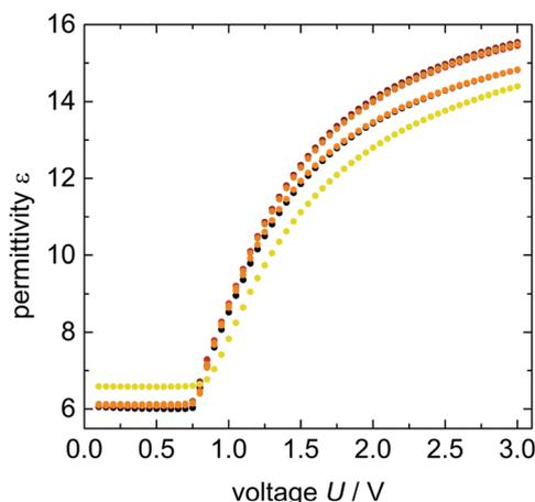
Fig. 8 Permittivity  $\epsilon$  as a function of electric field for 5CB (●) and 9OCB-PHMS@Fe<sub>3</sub>O<sub>4</sub> doped 5CB with different magnetic volume fraction  $\phi_m = 1.9 \times 10^{-5}$  (●),  $\phi_m = 9.4 \times 10^{-5}$  (●),  $\phi_m = 1.9 \times 10^{-4}$  (●),  $\phi_m = 4.7 \times 10^{-4}$  (●) and  $\phi_m = 9.4 \times 10^{-4}$  (●).
