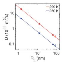
Fig. 3 The diffusion coefficient D versus the hydrodynamic radius  $R_h$  of the probe particles in water at the warmest (299 K) and coldest (260 K) measured temperature. Here we also include the PHF clusters (open circles). The hydrodynamic radius was determined by the Stokes-Einstein relation and macroscopic water viscosity at room temperature.
