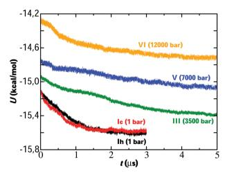
Fig. 2 Evolution of the potential energy as a function of time (on the microsecond time scale) obtained at  $\Delta T = -20$  K for the systems ice/ NaCl(ag) studied in this work.  $\Delta T$  is the difference between the melting temperature for each ice ( $T_{\rm m}$ ) using the TIP4P/2005 water model and the temperature of system studied (7). The pressure to which the direct coexistence simulations have been performed for each ice system is indicated in parentheses.
