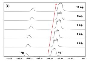
Fig. 7 (a) Selective 1D <sup>1</sup>H NOESY experiment. Protons of TMB were employed for selective excitation (green-labelled in the inset). Protons involved in the interaction are shown. Arrows qualitatively reflect the intensity of NOE. (b) Titration experiments monitoring the BF<sub>4</sub> anion by <sup>19</sup>F NMR.
