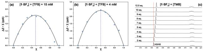
Fig. 6 Representative Job's plots for the interaction of compound 1 and TFB at (a) 15 mM in DMSO- $d_6$  and (b) 4 mM in acetone- $d_6$ : (c) <sup>1</sup>H NMR titration spectra (500 MHz) of 1.BF<sub>4</sub> (20 mM) with TMB in DMSO-d<sub>6</sub>. Key H3/H5 protons are labeled.
