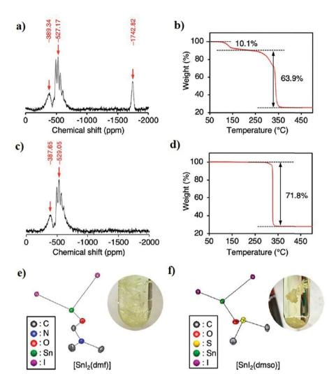
Fig. 2 Purified Snl<sub>2</sub> reagents, (a and b) <sup>119</sup>Sn MAS NMR spectra, and TGA analysis of commercially purchased Snl<sub>2</sub>. (c and d) <sup>119</sup>Sn MAS NMR spectra and TGA analysis of purified Snl<sub>2</sub> using the vacuum sublimation method. (e and f) Structural illustrations of [Snl<sub>2</sub>(DMF)] and [Snl<sub>2</sub>(DMSO)]. <sup>69</sup> Reproduced with permission Copyright 2020, American Chemical Society.
