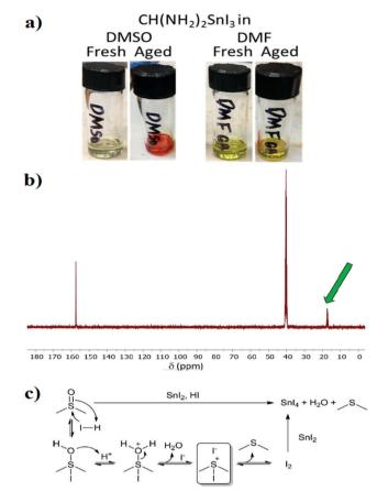
Fig. 3 Oxidative effect of DMSO, (a) FASnI<sub>3</sub> solutions in DMSO and DMF before and after ageing for 5 h at 120 °C.74 Reproduced with permission Copyright 2020, American Chemical Society. (b) Mechanism of Sn(II) oxidation by DMSO. (c) <sup>13</sup>C-NMR spectra of FASnI<sub>3</sub> heated at 100 °C for 30 min. The green arrow indicates the DMS-related peak.<sup>75</sup> Reproduced with permission, Copyright 2021, The Royal Society of Chemistry.
