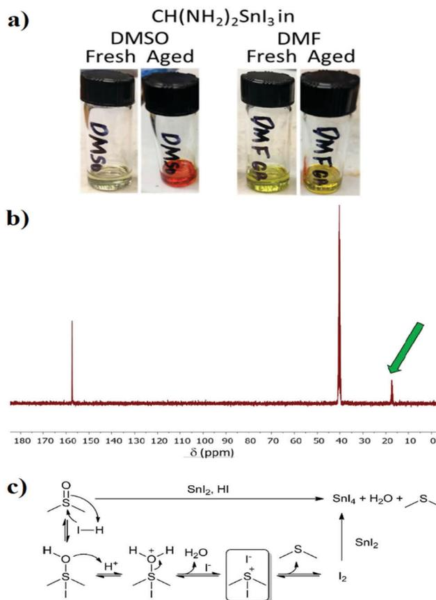
Fig. 3 Oxidative effect of DMSO. (a) FASnI<sub>3</sub> solutions in DMSO and DMF before and after ageing for 5 h at 120 °C.<sup>74</sup> Reproduced with permission Copyright 2020, American Chemical Society. (b) Mechanism of Sn(II) oxidation by DMSO. (c) <sup>13</sup>C-NMR spectra of FASnI<sub>3</sub> heated at 100 °C for 30 min. The green arrow indicates the DMS-related peak.<sup>75</sup> Reproduced with permission, Copyright 2021, The Royal Society of Chemistry.
