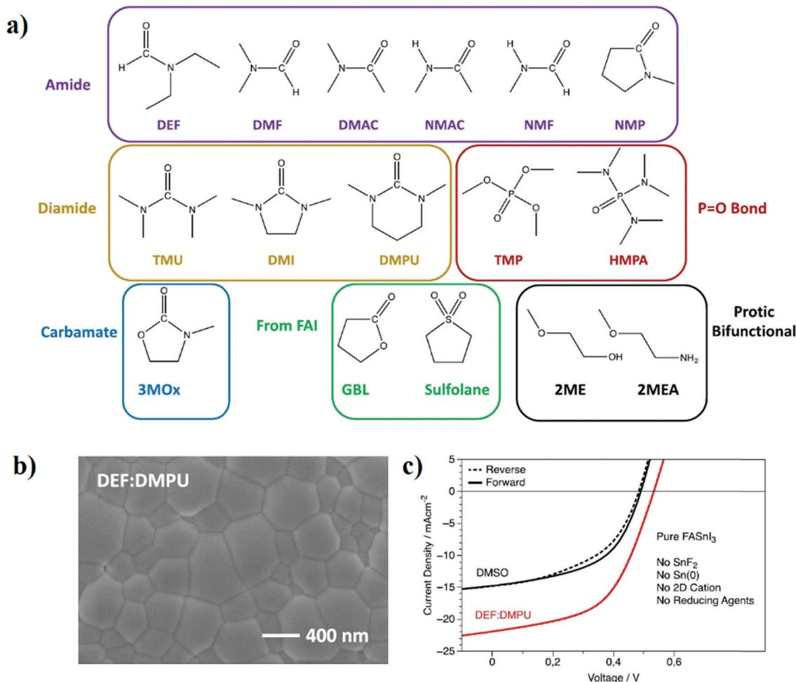
Fig. 4 (a) 16 nonsulfoxide solvents that formed stable perovskite solution divided into groups according to the functional group. (b) SEM images of the DEF:DMPU film. (c)  $J$ - $V$  curves of  $\text{FASnI}_3$  without any additives in DEF:DMPU against DMSO.<sup>78</sup> Reproduced with permission Copyright 2021, American Chemical Society.
