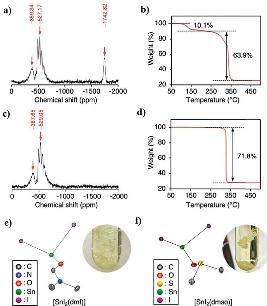
Fig. 2 Purified  $\text{SnI}_2$  reagents, (a and b)  $^{119}\text{Sn}$  MAS NMR spectra, and TGA analysis of commercially purchased  $\text{SnI}_2$ . (c and d)  $^{119}\text{Sn}$  MAS NMR spectra and TGA analysis of purified  $\text{SnI}_2$  using the vacuum sublimation method. (e and f) Structural illustrations of  $[\text{SnI}_2(\text{DMF})]$  and  $[\text{SnI}_2(\text{DMSO})]$ .<sup>69</sup> Reproduced with permission Copyright 2020, American Chemical Society.
