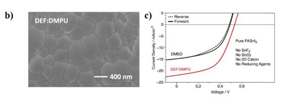
Fig. 4 (a) 16 nonsulfoxide solvents that formed stable perovskite solution divided into groups according to the functional group. (b) SEM images of the DEF:DMPU film. (c) J-V curves of FASnl<sub>3</sub> without any additives in DEF:DMPU against DMSO.<sup>78</sup> Reproduced with permission Copyright 2021, American Chemical Society
