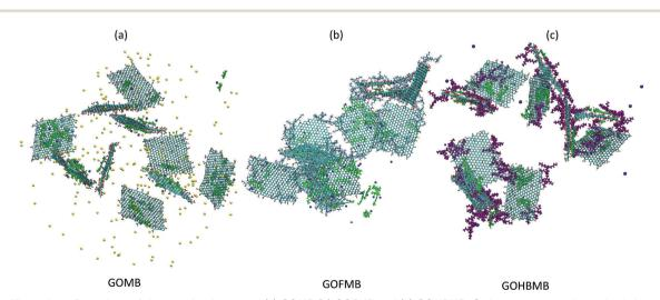
Fig. 3 Equilibrated configurations of the examined systems: (a) GOMB (b) GOFMB and (c) GOHBMB. Carbon atoms are shown in dark cyan, oxygen atoms in red and hydrogen atoms in white; yellow and blue beads correspond to the Na<sup>+</sup> and the Cl<sup>-</sup> counterions, respectively. The free BPEI molecules in the GOHBMB system are shown in purple. Water molecules are not shown for clarity
