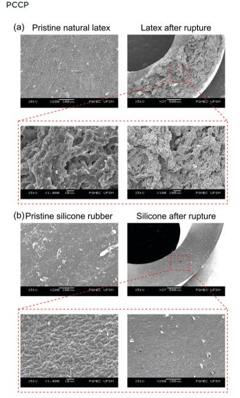
Fig. 6 SEM micrographs of the (a) natural latex and (b) silicone rubber before and after fatigue tests at different magnifications.
