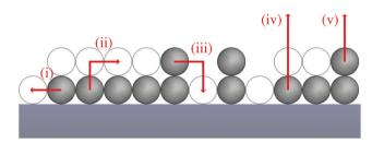
Fig. 1 Schematic representation of the simple chain geometry and elementary processes. The displayed processes are diffusion (i), layer exchange from the first to the second (ii) and from the second to the first layer (iii) as well as desorption from the first (iv) and second (v) layer. Occupied adsorption sites are displayed as filled spheres, while unoccupied adsorption sites are shown as empty spheres.
