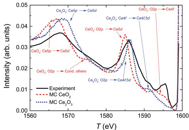
Fig. 9 Comparison between the REEL spectra of bulk  $\text{CeO}_2$  (red line) and  $\text{Ce}_2\text{O}_3$  (blue line) simulated by MC compared with the directly measured spectrum (black line).<sup>21</sup> Spectra are normalized with respect to the area under the curves. Zero-loss peak is found at the extreme right of the spectrum. The primary beam impinges the material with an incident angle equal to  $60^\circ$  with respect to the surface's normal.
