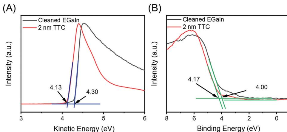
Fig. 5 (A) The SECO and (B) VB spectra for a clean  $\text{GaO}_x/\text{EGaIn}$  film (black) and after deposition of 2 nm TTC (red). The cut-off positions and HOMO or VB onsets are marked with blue and green bars, respectively. The  $\Phi$  and HOMO or VB onset energies are denoted alongside.
