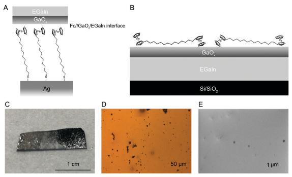
Fig. 1 (A) Schematic illustration of the  $Ag-S(CH_2)_{11}Fc \|GaO_x/EGaIn\|$  junction and (B) of the  $Fc-(CH_2)_{14}-Fc$  deposited on a layer of  $GaO_x/EGaIn\|$  on a Si/SiO<sub>2</sub> substrate. (C) A photograph, (D) an optical microscopy image, and (E) a scanning electron microscopy image, of the GaO<sub>x</sub>/EGaIn film.
