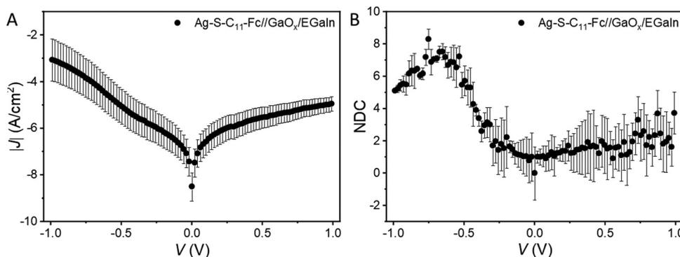
Fig. 6 (A) Shows an average of  $|J|$  vs.  $V$  measurement on an  $\text{Ag-S-C}_{11}\text{-Fc//GaO}_x/\text{EGaIn}$  molecular diode, which is subsequently smoothed by a moving smoothing function to obtain the derivative which is used to obtain the (B) NDC plot for the measurement, error bar: standard deviation for 5 scans.
