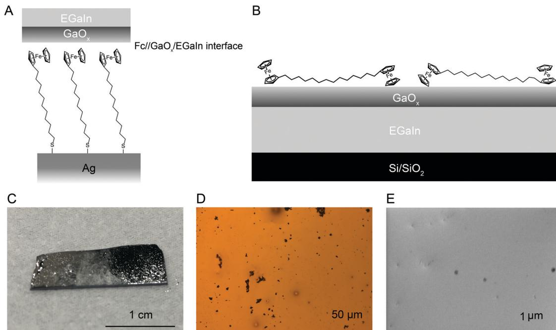
Fig. 1 (A) Schematic illustration of the Ag–S(CH<sub>2</sub>)<sub>11</sub>Fc||GaO<sub>x</sub>/EGaIn junction and (B) of the Fc–(CH<sub>2</sub>)<sub>14</sub>–Fc deposited on a layer of GaO<sub>x</sub>/EGaIn on a Si/SiO<sub>2</sub> substrate. (C) A photograph, (D) an optical microscopy image, and (E) a scanning electron microscopy image, of the GaO<sub>x</sub>/EGaIn film.
