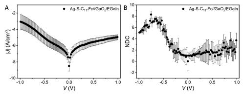
Fig. 6 (A) Shows an average of |J| vs. V measurement on an Ag-S-C<sub>11</sub>-Fc $\|$ GaO $_x$ /EGaIn molecular diode, which is subsequently smoothened by a moving smoothening function to obtain the derivative which is used to obtain the (B) NDC plot for the measurement, error bar: standard deviation for 5 scans.
