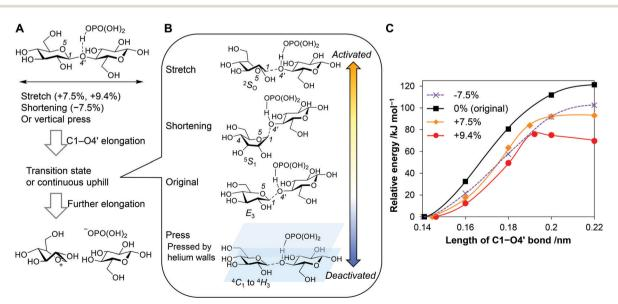
Fig. 6 Scission of glycosidic bond of cellobiose in the presence of forces. (A) Schematic of the reaction. (B) Structures at transition or the transient states. (C) Potential curves as a function of C1-O4' bond length for the stretched or shortened molecule. H<sub>3</sub>PO<sub>4</sub> coordinates on O4' of cellobiose as an acid catalyst.
