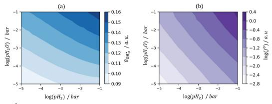
Fig. 6  $\theta_{OH_{O}^{\bullet}}$  (a) and  $f^{0}$  (b) at the Sm<sub>0.2</sub>Ce<sub>0.8</sub>O<sub>1.9</sub>-gas interface as a function of steam and hydrogen partial pressure at 500 °C.
