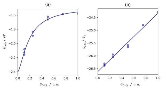
Hydroxyl coverage dependence on (a) adsorption enthalpy fit to (15) and (b) adsorption entropy with linear fitting
