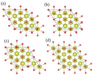
Fig. 2 Structure of lowest energy ceria after surface relaxation. (a)  $\theta_{\mathrm{OH}_{0}^{\bullet}}$ 0.25 with a polaron positioned as the nearest neighbour (NN) with respect to the hydroxyl, (b)  $\theta_{\mathrm{OH}_{\mathrm{O}}^{\bullet}}=0.50$  with polarons positioned NN with respect to the hydroxyls, (c)  $\theta_{\rm OH_O^{\bullet}}=0.75$  and (d)  $\theta_{\rm OH_O^{\bullet}}=1.00$ . Ce, O and H atoms are shown as yellow, red and white, respectively
