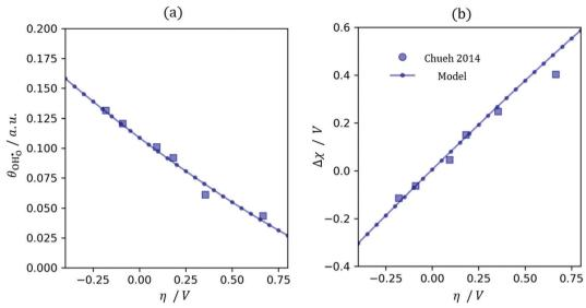
Fig. 5  $\theta_{OH_{0}^{\bullet}}$  (a) and  $\chi$  (b) on a Sm<sub>0.2</sub>Ce<sub>0.8</sub>O<sub>1.9</sub>-gas interface as a function of overpotential at 500 °C in 1:8:4 H<sub>2</sub>O:H<sub>2</sub>:Ar. Squares represent data collected by APXPS measurements (Chueh *et al.*).<sup>29</sup> The dotted and filled lines represent the numerical and analytical solutions to (12), respectively.
