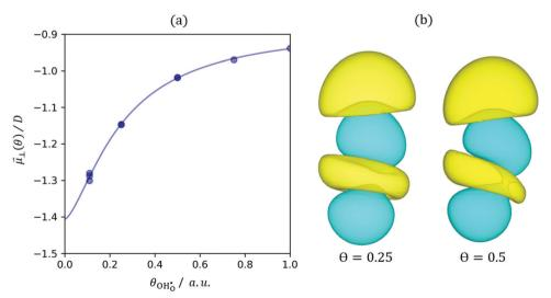
Fig. 3 (a) Calculated hydroxyl dipole moment normal to the ceria[111] termination as a function of coverage. The line fits to egn (13). (b) Charge density difference isosurface (0.005 Bohr<sup>-3</sup>) of the hydroxyl on the ceria surface where negative and positive charge density is represented by blue and yellow isosurfaces, respectively. O site bottom and H site top
