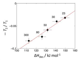
Fig. 5 Direct comparison of NMR and TPD data for pyridine adsorbed within HZSM-5 zeolites with varying silica/alumina rations (SAR). The red line is a linear fit to the data. SAR values are indicated above each data point.
