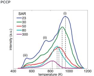
Fig. 3 Mass-normalised TPD spectra of pyridine in HZSM-5 with varying silica/alumina ratios (SAR) acquired with a heating rate of 10 K min<sup>-1</sup>. Dashed lines indicate the position of the maximum desorption rate for each material.
