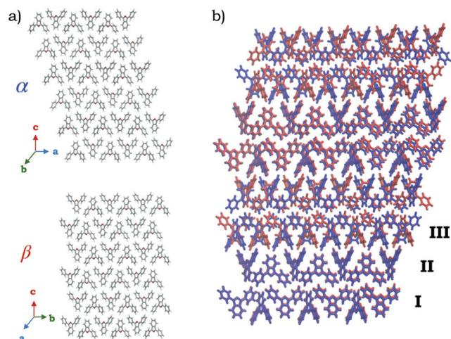
Fig. 7 The two polymorphs of DPBF. (a) The long-range packing of the  $\alpha$  and  $\beta$  forms are depicted. Vector lengths are indicated in each polymorph. (b) Superposition of a portion of the  $\alpha$  (blue) and  $\beta$  (red) polymorphs. Nearest-neighbours are almost identical (rows I and II) whereas next-nearest are different (row III).
