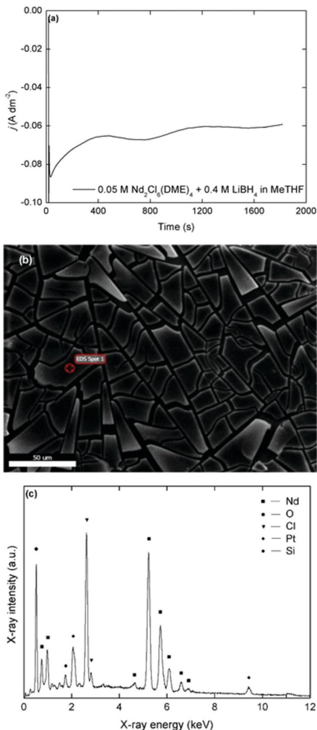
Fig. 7 (a) Plot of the current density versus time for a potentiostatic deposition at  $-3.3$  V vs.  $\text{Fc}^+/\text{Fc}$  for 1800 s in a stirred solution of  $0.05 \text{ mol L}^{-1} \text{Nd}_2\text{Cl}_6(\text{DME})_4 + 4$  molar equivalents of  $\text{LiBH}_4$  in MeTHF. (b) Scanning electron micrograph of the deposit at X500 magnification. (c) EDX spectrum of the deposit in the energy range 0–12 keV, recorded at an acceleration voltage of 20 kV with assignment of the major lines.
