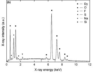
Fig. 6 (a) SEM micrograph of a dysprosium deposit, prepared at  $-3.1 \,\mathrm{V}$  vs. Fc<sup>+</sup>/Fc for 1800 s on a platinum-coated silicon wafer substrate in a stirred solution of 0.1 mol  $L^{-1}$  Dy(Tf<sub>2</sub>N)<sub>3</sub> + 4 molar equivalents of NaBH<sub>4</sub> in DME. (b) EDX spectrum of the deposit in the energy range 0-12 keV, recorded at an acceleration voltage of 20 kV with assignment of the major lines
