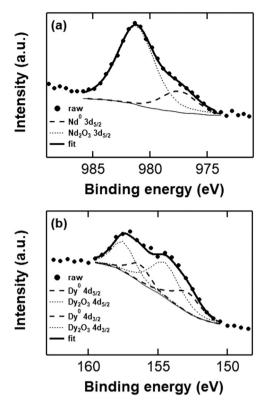
Fig. 8 Curve-fitted Nd 3d<sub>5/2</sub> (a) and Dy 4d (b) XPS spectra (surface) from deposits with a thickness of approx. 1 µm, obtained from potentiostatic deposition in Nd(Tf<sub>2</sub>N)<sub>3</sub> or Dy(Tf<sub>2</sub>N)<sub>3</sub> + TBABH<sub>4</sub> electrolytes at  $-3.4 \text{ V vs. Fc}^+$ /Fc.
