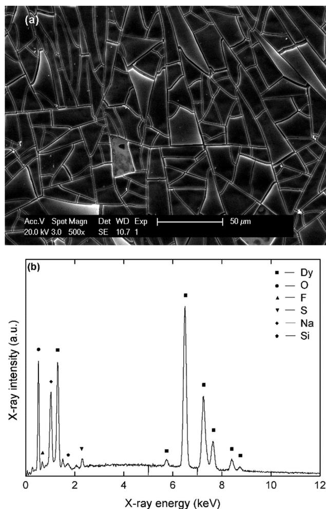
Fig. 6 (a) SEM micrograph of a dysprosium deposit, prepared at  $-3.1$  V vs.  $\text{Fc}^+/\text{Fc}$  for 1800 s on a platinum-coated silicon wafer substrate in a stirred solution of  $0.1 \text{ mol L}^{-1} \text{ Dy}(\text{Tf}_2\text{N})_3 + 4$  molar equivalents of  $\text{NaBH}_4$  in DME. (b) EDX spectrum of the deposit in the energy range 0–12 keV, recorded at an acceleration voltage of 20 kV with assignment of the major lines.
