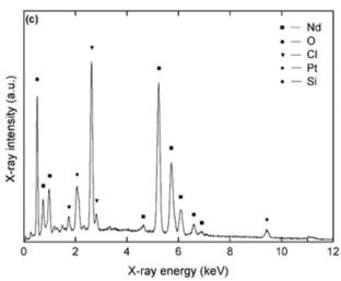
Fig. 7 (a) Plot of the current density versus time for a potentiostatic deposition at -3.3 V vs. Fc+/Fc for 1800 s in a stirred solution of 0.05 mol  $L^{-1}$  Nd<sub>2</sub>Cl<sub>6</sub>(DME)<sub>4</sub> + 4 molar equivalents of LiBH<sub>4</sub> in MeTHF. (b) Scanning electron micrograph of the deposit at X500 magnification. (c) EDX spectrum of the deposit in the energy range 0-12 keV, recorded at an acceleration voltage of 20 kV with assignment of the major lines
