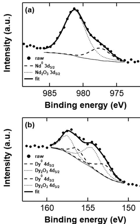
Fig. 8 Curve-fitted  $\text{Nd } 3d_{5/2}$  (a) and  $\text{Dy } 4d$  (b) XPS spectra (surface) from deposits with a thickness of approx.  $1 \mu\text{m}$ , obtained from potentiostatic deposition in  $\text{Nd}(\text{Tf}_2\text{N})_3$  or  $\text{Dy}(\text{Tf}_2\text{N})_3 + \text{TBABH}_4$  electrolytes at  $-3.4$  V vs.  $\text{Fc}^+/\text{Fc}$ .
