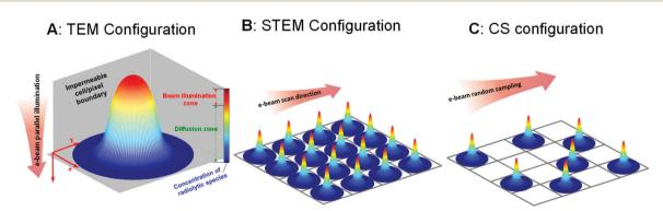
Fig. 1 Schematic illustration of the electron/liquid interaction zones that arise in electron microscopy when (A) a single large illumination spot is contained within a chemically-inert and impermeable boundary, (B) multiple pixels are involved, (C) random-sampling scheme is applied, e.g. compressive sensing mode
