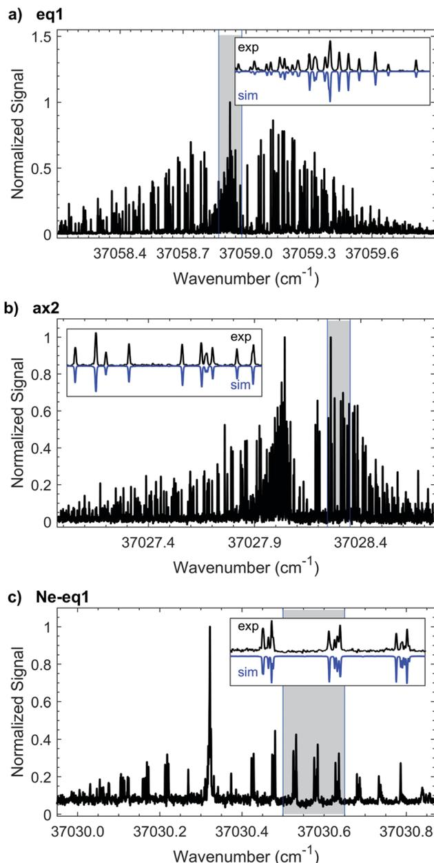
Fig. 4 HR-LIF spectra of 3 species of 1-indanol: (a) conformer eq1 recorded at  $\sim 1$  K, (b) conformer ax2 recorded at  $\sim 1.5$  K, and (c) neon complex Ne-eq1 recorded at  $\sim 1.5$  K. In the insets the blue traces show the simulated spectra and the black traces are experimental data. These insets correspond to the domains shadowed with grey. These spectra were recorded at a scan rate of  $\sim 5$  MHz per second.
