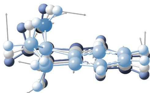
**Fig. 5** Normal mode associated with the  $+116 \text{ cm}^{-1}$  band. The displacement of the vibration is shown with grey arrows. The overlaid molecular structures depict various stages of the vibration.
