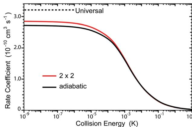
Fig. 7 The total rate coefficient is plotted as function of collision energy for the  $\text{Li} + \text{LiNa}(v = 0, j = 0) \rightarrow \text{Li}_2 + \text{Na}$  reaction. The red and black curves correspond to the coupled two-state diabatic ( $2 \times 2$ ) and single surface adiabatic (NGP) calculations, respectively. The horizontal black dashed line denotes the ultracold rate coefficient computed using a universal model.
