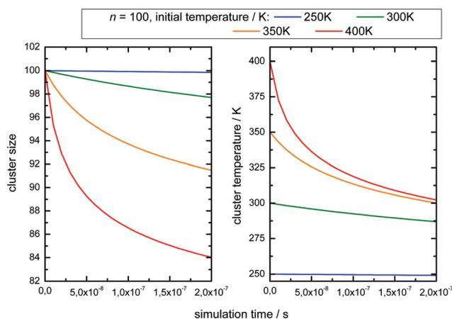
Fig. 6 Simulation of monomer loss (left panel) and temperature drop (right panel) of  $(\text{H}_2\text{O})_{100}$  over 200 ns as a function of starting temperature. The sizes and temperature are weighted means of the distribution.
