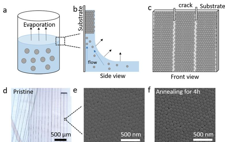
**Fig. 1** (a–c) Scheme of the fiber preparation. (a) Evaporation of a suspension of silica nanoparticles in ethanol/water. (b) Self-assembly of SiO<sub>2</sub> NPs on the vial wall driven by the capillary and Marangoni flows. (c) Directed and uniform development of cracks accompanying the drying of the solvent. (d and e) Optical and SEM images of pristine fibers. (f) SEM image of the annealed fiber, treated at  $T = 1173$  K for 4 h.
