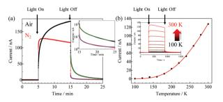
Fig. 3 (a) Photocurrent and persistent photocurrent responses of the TIPS-Pn film for light illumination using the Xe lamp in air (black curve) and under a N<sub>2</sub> atmosphere (red curve) at room temperature. Inset is the decay of the persistent photocurrent depicted using a log scale for the vertical axis. (b) Temperature dependence of the photocurrent response under a N<sub>2</sub> atmosphere
