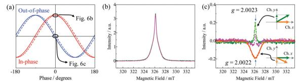
Fig. 6 (a) Model of an output function of the reference signal phase for an EDMR signal. The red and blue curves show in-phase (channel x) and out-ofphase (channel y) signals, respectively. (b) Reference signal phase dependence of in-phase EDMR spectra under the N2 atmosphere at 200 K. (c) Reference signal phase dependence of the out-of-phase EDMR spectra.
