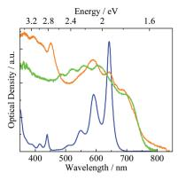
Fig. 2 UV-vis optical density spectrum of TIPS-Pn absorption in CH<sub>2</sub>Cl<sub>2</sub> solution (blue curve), transmission spectrum of the TIPS-Pn film (orange curve), and diffuse reflectance spectrum of ground powder of the TIPS-Pn sample (green curve).
