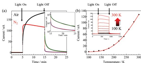
Fig. 3 (a) Photocurrent and persistent photocurrent responses of the TIPS-Pn film for light illumination using the Xe lamp in air (black curve) and under a  $\text{N}_2$  atmosphere (red curve) at room temperature. Inset is the decay of the persistent photocurrent depicted using a log scale for the vertical axis. (b) Temperature dependence of the photocurrent response under a  $\text{N}_2$  atmosphere.
