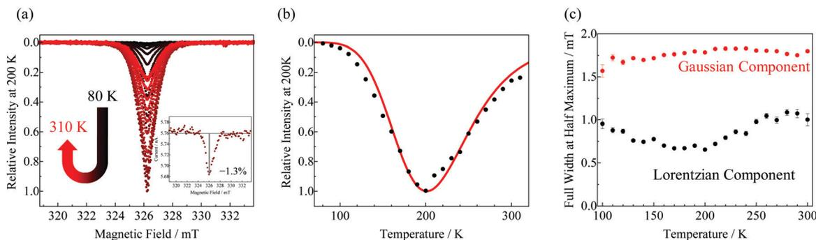
Fig. 5 (a) Temperature dependence of the photocurrent-detected EDMR spectra of the VVD film of TIPS-Pn under the  $N_2$  atmosphere. (b) Temperature dependence of the integral signal intensity (black dots) and the simulation curve using eqn (S52) ( $ESI^\dagger$ ) (red curve). (c) Temperature dependence of linewidth for Gaussian component to Lorentzian one. The black circles and red circles show Lorentz and Gaussian analysed by eqn (5).
