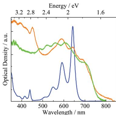
Fig. 2 UV-vis optical density spectrum of TIPS-Pn absorption in  $\text{CH}_2\text{Cl}_2$  solution (blue curve), transmission spectrum of the TIPS-Pn film (orange curve), and diffuse reflectance spectrum of ground powder of the TIPS-Pn sample (green curve).
