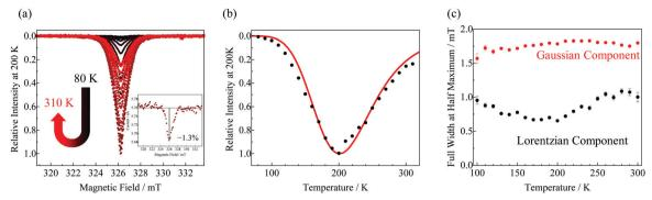
Fig. 5 (a) Temperature dependence of the photocurrent-detected EDMR spectra of the VVD film of TIPS-Pn under the N<sub>2</sub> atmosphere. (b) Temperature dependence of the integral signal intensity (black dots) and the simulation curve using egn (S52) (ESI†) (red curve). (c) Temperature dependence of linewidth for Gaussian component to Lorentzian one. The brack circles and red circles show Lorentz and Gaussian analysed by eqn (5)
