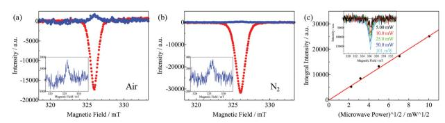
Fig. 4 EDMR spectra of TIPS-Pn through monitoring of the photocurrent (red curve) and the persistent photocurrent (blue curve) at room temperature under (a) air and (b) N2 atmosphere. (c) Photocurrent-detected EDMR spectra of the VVD-prepared TIPS-Pn film as a function of microwave power at 80 K under the N<sub>2</sub> atmosphere.
