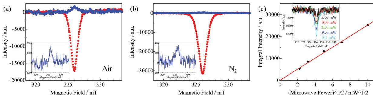
Fig. 4 EDMR spectra of TIPS-Pn through monitoring of the photocurrent (red curve) and the persistent photocurrent (blue curve) at room temperature under (a) air and (b)  $\text{N}_2$  atmosphere. (c) Photocurrent-detected EDMR spectra of the VVD-prepared TIPS-Pn film as a function of microwave power at 80 K under the  $\text{N}_2$  atmosphere.
