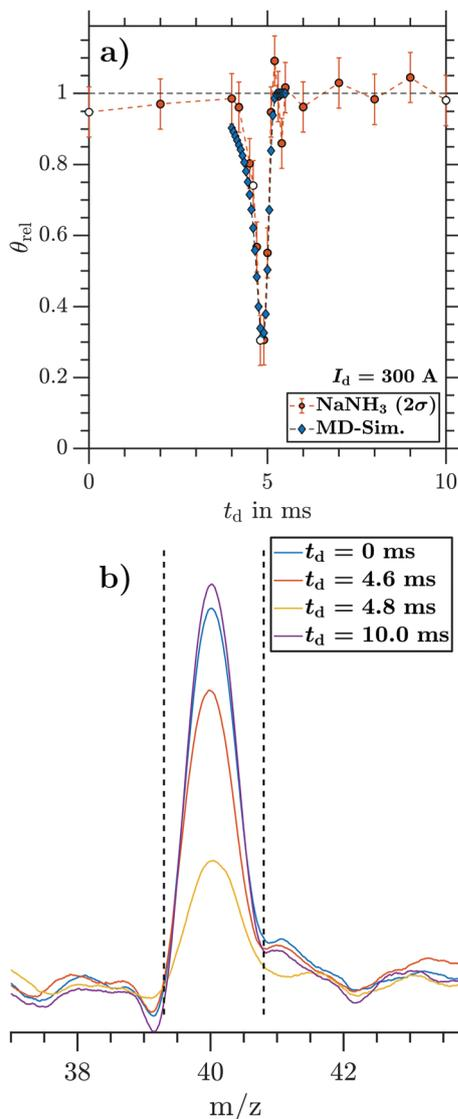
**Fig. 6** (a) Relative integrated NaNH<sub>3</sub> TOF signal  $\theta_{rel}$  (2000 shots per data point) as a function of  $t_d$  (circles with  $2\sigma$  error), compared with MD simulations (diamonds). (b) NaNH<sub>3</sub> TOF signals for four representative  $t_d$  corresponding to the open black circles at 0, 4.6, 4.8 and 10.0 ms in panel a. The deflector was operated at  $I_d = 300$  A.
