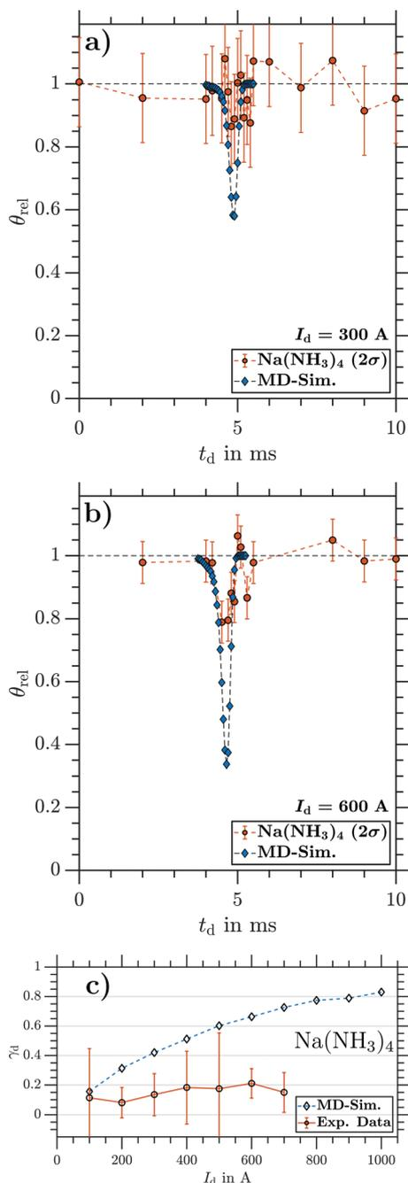
Fig. 10  $\theta_{rel}$  as a function of  $t_d$  of  $\text{Na}(\text{NH}_3)_4$  recorded at (a)  $I_d = 300$  A and (b)  $I_d = 600$  A. (c) Maximal  $\gamma_d$  as a function of  $I_d$  for  $\text{Na}(\text{NH}_3)_4$ . Circles: experiment. The error indicates  $2\sigma$ . Diamonds: MD simulation.
