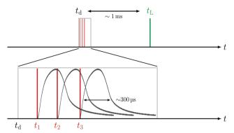
Fig. 2 Sketch of the timing sequence of a deflection measurement. The relative timing between deflection ( $t_d$ ) and ionization ( $t_L$ ) is varied for various TOF measurements (upper sketch). The deflector consists of three individual coils, which can be operated with different offset timings  $(t_1, t_2, t_3)$  $t_3$ ) relative to  $t_d$ . The lower sketch shows the experimentally measured magnetic field pulses ( $I_d$  = 300 A) for each coil timing,  $t_1$ ,  $t_2$ , and  $t_3$ .
