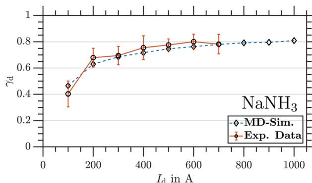
**Fig. 7** Maximal  $\gamma_d$  as a function of  $I_d$  for NaNH<sub>3</sub>. Circles: experiment. The error indicates  $2\sigma$ . Diamonds: MD simulation. The deflector was operated in a  $t_1 < t_2 < t_3$  coil timing sequence.
