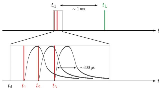
Fig. 2 Sketch of the timing sequence of a deflection measurement. The relative timing between deflection ( $t_d$ ) and ionization ( $t_L$ ) is varied for various TOF measurements (upper sketch). The deflector consists of three individual coils, which can be operated with different offset timings ( $t_1$ ,  $t_2$ ,  $t_3$ ) relative to  $t_d$ . The lower sketch shows the experimentally measured magnetic field pulses ( $I_d = 300$  A) for each coil timing,  $t_1$ ,  $t_2$ , and  $t_3$ .
