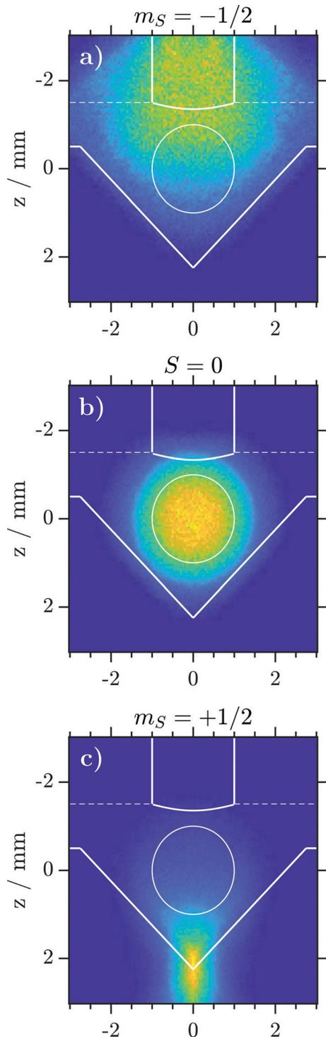
Fig. 4 MD simulations of a particle with the same mass as  $\text{NaNH}_3$  for spin states (a)  $m_S = -1/2$ , (b)  $S = 0$  and (c)  $m_S = +1/2$ .  $10^6$  trajectories were calculated for all simulations. The white lines indicate the cross section of the flight channel, while the white dotted lines represent the borders of the epoxy layers. The white circle represents the detection skimmer.
