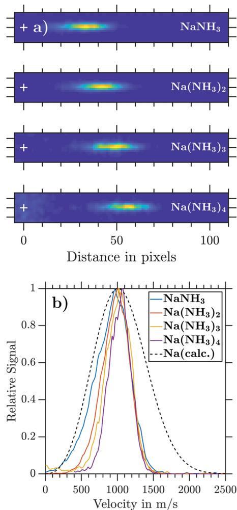
Fig. 3 (a) Na(NH<sub>3</sub>)<sub>n</sub> ( $n = 1-4$ ) ion images measured in perpendicular extraction at  $V_R = 7$  kV. (b) Experimental Na(NH<sub>3</sub>)<sub>n</sub> velocity distributions retrieved from ion images. The calculated velocity distribution for an effusive Na-beam at 265 °C is shown as a dashed line (see the ESI,† Section S3). Its distribution function is given by the convolution of a 1D Maxwell–Boltzmann distribution with an exponential transmission function.
