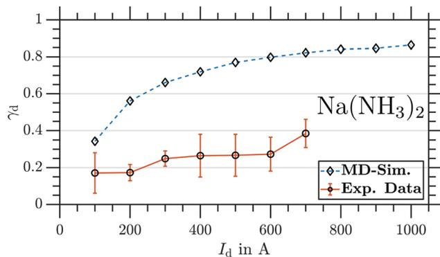
Fig. 8 Maximal  $\gamma_d$  as a function of  $I_d$  for  $\text{Na}(\text{NH}_3)_2$ . Circles: experiment. The error indicates  $2\sigma$ . Diamonds: MD simulation. The deflector was operated in a  $t_1 < t_2 < t_3$  coil timing sequence.
