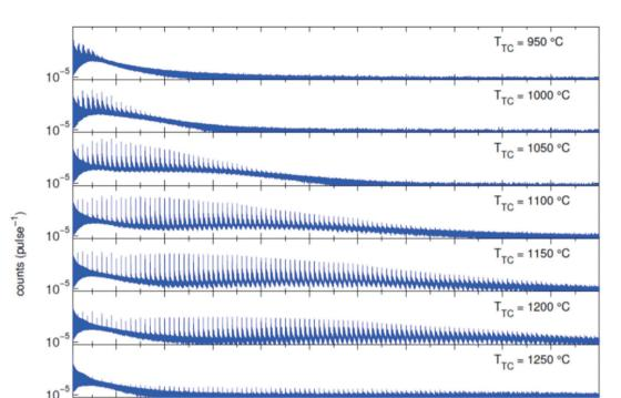
Fig. 2 Mass spectra of an Au doped He droplet beam ( $T_0 = 9$  K and  $p_0 = 20$  bar,  $N_{\rm He} \approx 1.8 \times 10^6$ ) for different oven temperatures  $T_{\rm TC}$ . Additional peaks appear due to the adsorption of water molecules in the pickup chamber.  $^{70}$
