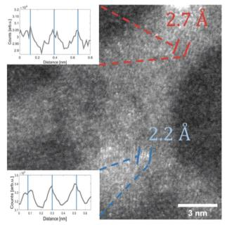
Fig. 17 STEM HAADF image of a V<sub>2</sub>O<sub>5</sub> particle (synthesised at 5.4 K cold head temperature). Two regions are marked where lattice constants could be extracted from the image. The respective intensity profile between the lines is shown in the inset. The black lines indicate a group of planes with a spacing of 2.7 Å the blue lines mark a group of planes with a spacing of 2.2 Å. Ref. 128 - reprinted with permission of the PCCP Owner Societies.
