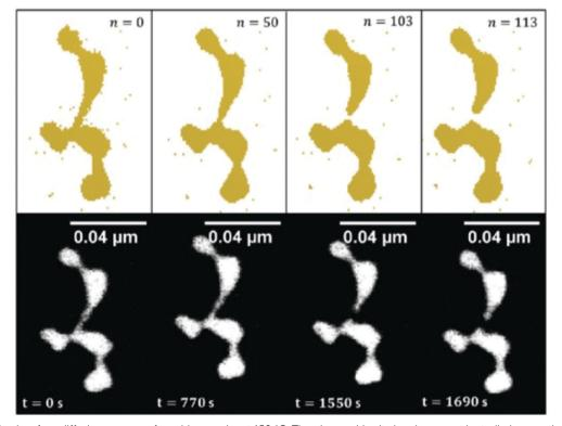
Fig. 11 Time evolved surface diffusion process of a gold nanowire at 150 °C. The observed in situ breakup event is studied over a time period of nearly half an hour (lower images) and are compared to the results obtained with the CA (upper images) in order to draw a fit between iteration steps and experimental observation time. Ref. 101 - reprinted with permission of the PCCP Owner Societies.
