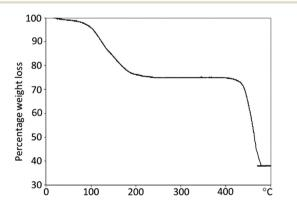
Fig. 6 Thermogravimetric analysis of 24 h sample of MIL-68(In), showing 25 and 37% weight loss at different temperatures, corresponding to loss of adsorbed organic species from the specimen, followed by the decomposition of MIL-68(In) to indium oxide, carbon dioxide, and water.
