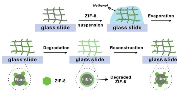
**Fig. 1** Schematic illustration of the degradation–reconstruction process of ZIF-8 loaded on various fibres.
