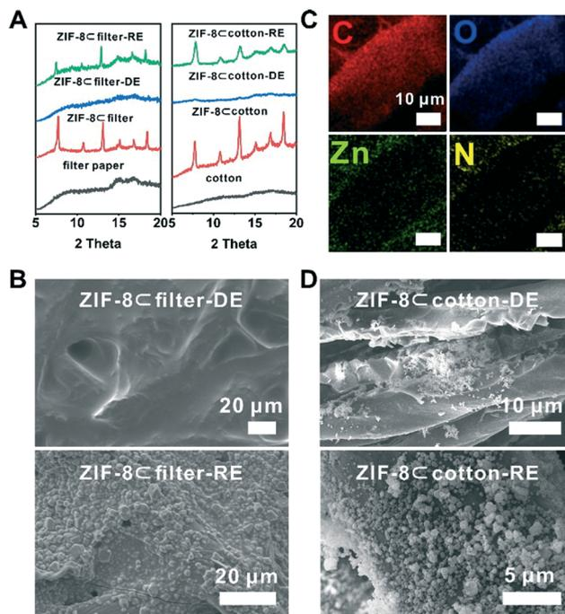
**Fig. 3** (A) PXRD patterns of the degradation–reconstruction processes of ZIF-8  $\subset$  filter and ZIF-8  $\subset$  cotton; SEM images of (B) ZIF-8  $\subset$  filter after degradation and reconstruction and (D) ZIF-8  $\subset$  cotton after degradation and reconstruction; (C) EDS elemental mapping images of ZIF-8  $\subset$  filter after degradation.
