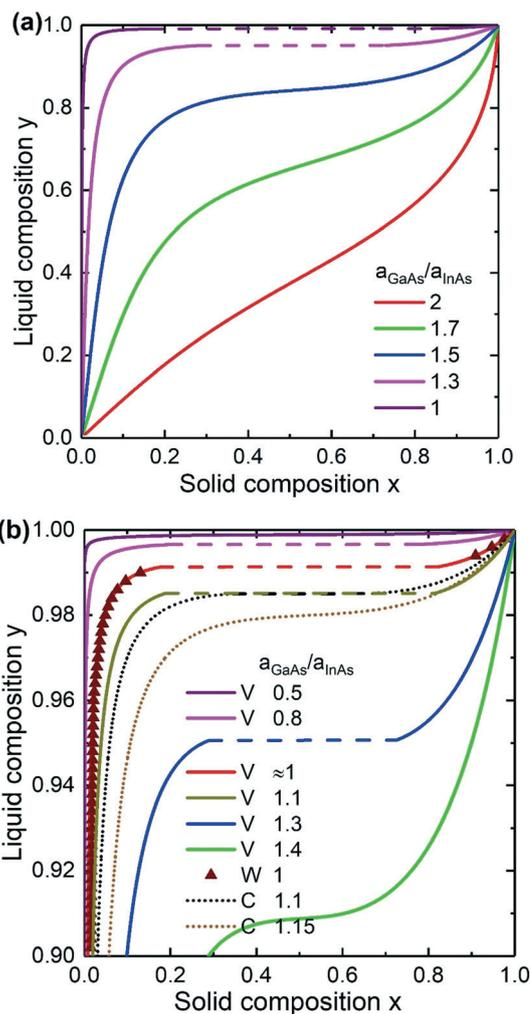
**Fig. 4** Liquid–solid composition dependences of InGaAs alloy for different surface energy ratio calculated within the Vegard model (a) and within Vegard (V), Wilemski (W) and convex (C) models (b). Triangles correspond to the Wilemski approach. The solid curves are the Vegard's law case and dots are the convex model with  $\alpha = 0.5$ . The dashed lines correspond to the miscibility gap.
