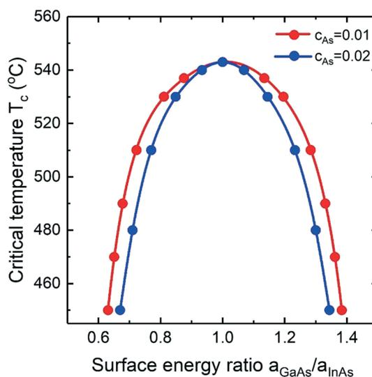
Fig. 7 Critical temperature versus the ratio of binary surface energy terms for InGaAs materials system at fixed As concentration of  $c_{\text{As}} = 0.01$  (red curve) and  $c_{\text{As}} = 0.02$  (blue curve). The dots represent numerical calculations and the solid curves are polynomial fits.
