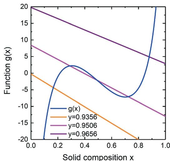
**Fig. 3** Illustration of the  $y(x)$  selection rule for InGaAs materials system. The blue solid curve is  $g(x)$  function; the tilted lines are  $f(y) + u(y)x$  calculated for different  $y$  and at fixed  $a_{\text{GaAs}}/a_{\text{InAs}} = 1.3$ .
