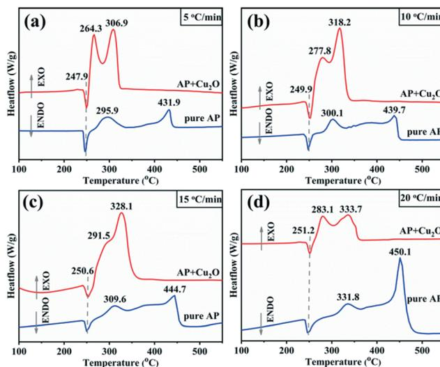
Fig. 7 DSC thermographs of AP and the mixture of AP with  $\text{Cu}_2\text{O}$  at different heating rates: (a) 5 °C  $\text{min}^{-1}$ ; (b) 10 °C  $\text{min}^{-1}$ ; (c) 15 °C  $\text{min}^{-1}$ ; (d) 20 °C  $\text{min}^{-1}$ .
