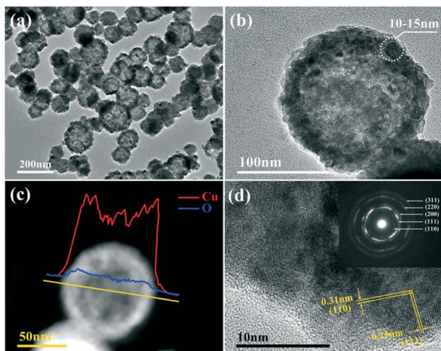
**Fig. 2** (a) Low magnification TEM image of the  $\text{Cu}_2\text{O}$  hollow spheres; (b) TEM image of a single  $\text{Cu}_2\text{O}$  hollow sphere; (c) corresponding EDX line scan; (d) HRTEM image (inset: SAED image).
