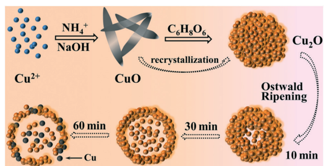
Fig. 5 Schematic diagram of the formation process of \text{Cu}_2\text{O} hollow spheres.
