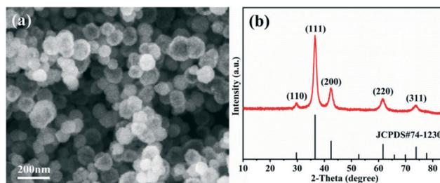
Fig. 1 (a) The SEM image and (b) XRD pattern of the synthesized Cu<sub>2</sub>O hollow spheres.
