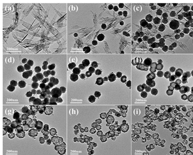
**Fig. 3** TEM images of the samples with different reaction times: (a) after 5 min of adding NaOH; (b) after adding AA and reacting for 10 s; (c) 1 min; (d) 5 min; (e) 10 min; (f) 20 min; (g) 30 min; (h) 60 min; (i) 120 min.
