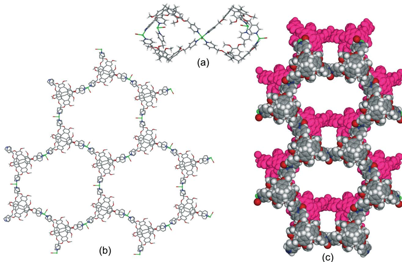
**Fig. 8** Crystal structure of  $[\text{Cu}_3(\text{L}3)_4(\text{H}_2\text{O})_3] \cdot 6(\text{OTf}) \cdot n(\text{DMSO})$ . (a) Two  $\text{Cu}_3\text{L}_2$  capsules linked through a shared  $\text{Cu}(\text{II})$ -vertex; (b) 2D network of linked capsules; (c) packing of two network layers (one in pink) showing substantial channels with largest ca.  $1.5 \times 3$  nm cross-section.<sup>20</sup>
