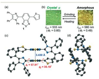
Fig. 1 (a) Molecular structure of 1. (b) Photographs of the MCL of  $1-\alpha$ ( $\lambda_{ex}$  = 365 nm). (c) Front view and (d) side view of 1- $\alpha$  for the two molecules in spatial proximity with thermal ellipsoids at 50% probability. All hydrogen atoms are omitted for clarity. Color code: gray = C; blue = N; yellow = S.
