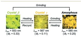
Fig. 5 Photographs of the mechanical and thermal stimuli-responsive emission color change of 1- $\beta$  and the MCL of 1- $\gamma$  ( $\lambda_{ex}$  = 365 nm).
