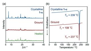
Fig. 2 (a) PXRD patterns and (b) DSC thermograms for the MCL of 1- $\alpha$ . The  $T_{\rm m}$  and  $T_{\rm c}$  values are noted near the corresponding peaks.
