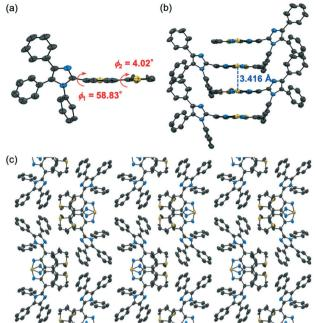
Fig. 7 (a) Molecular structure of  $1-\gamma$ . (b) Intermolecular stacking structure of  $1-\gamma$ . (c) Packing structure of  $1-\gamma$  viewed along the c-axis. Thermal ellipsoids at 50% probability. All hydrogen atoms are omitted for clarity. Color code: gray = C; blue = N; yellow = S.
